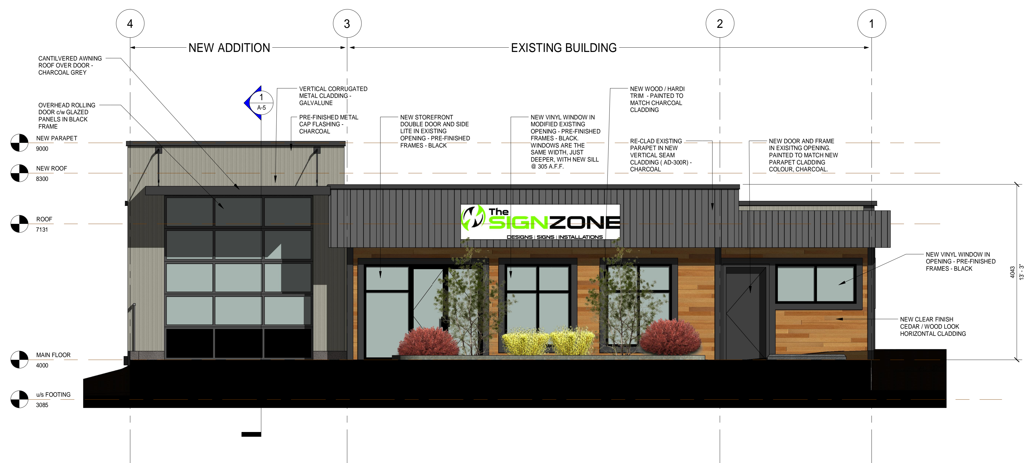
1 NORTH ELEVATION ( SHENTON ROAD ) 1 : 50
